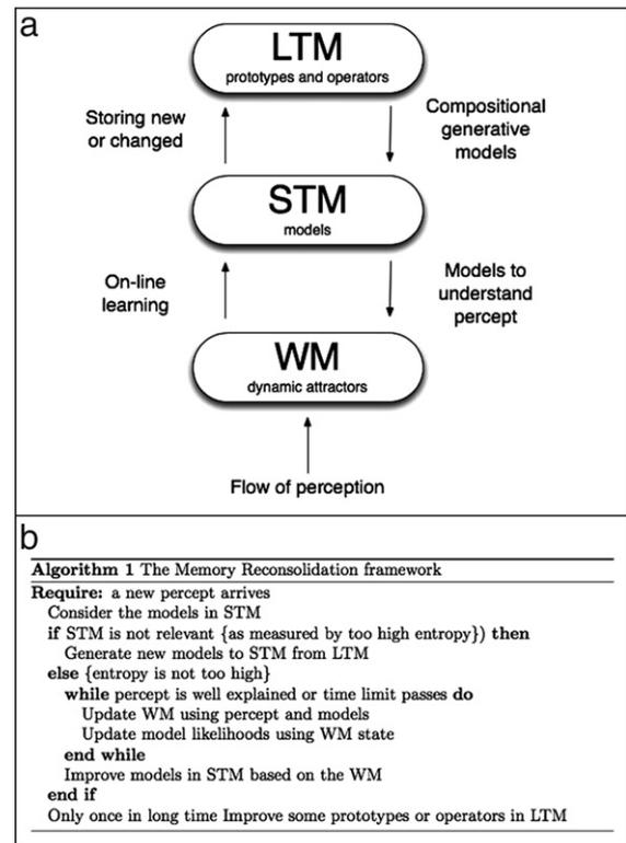
Fig. 5. Algorithmic view of memory system: (a) The figure depicts Long Term Memory that includes prototypes (e.g., ball, red) and operators (e.g., association) that together can form instances or models that are deposited into Short Term Memory. Short Term Memory's models can be updated by Working Memory via the RAN update algorithm. Working Memory hosts the state nodes of the RAN and enables the perception of new inputs. (b) The algorithm associated with the proposed framework of memory.
